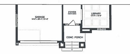
PARTIAL FIRST FLOOR PLAN FOR ELEV. 'OLIVIA' NOTE - PARTIAL PLANS TO BE READ IN CONJUNCTION W/COMPLETE PLANS
