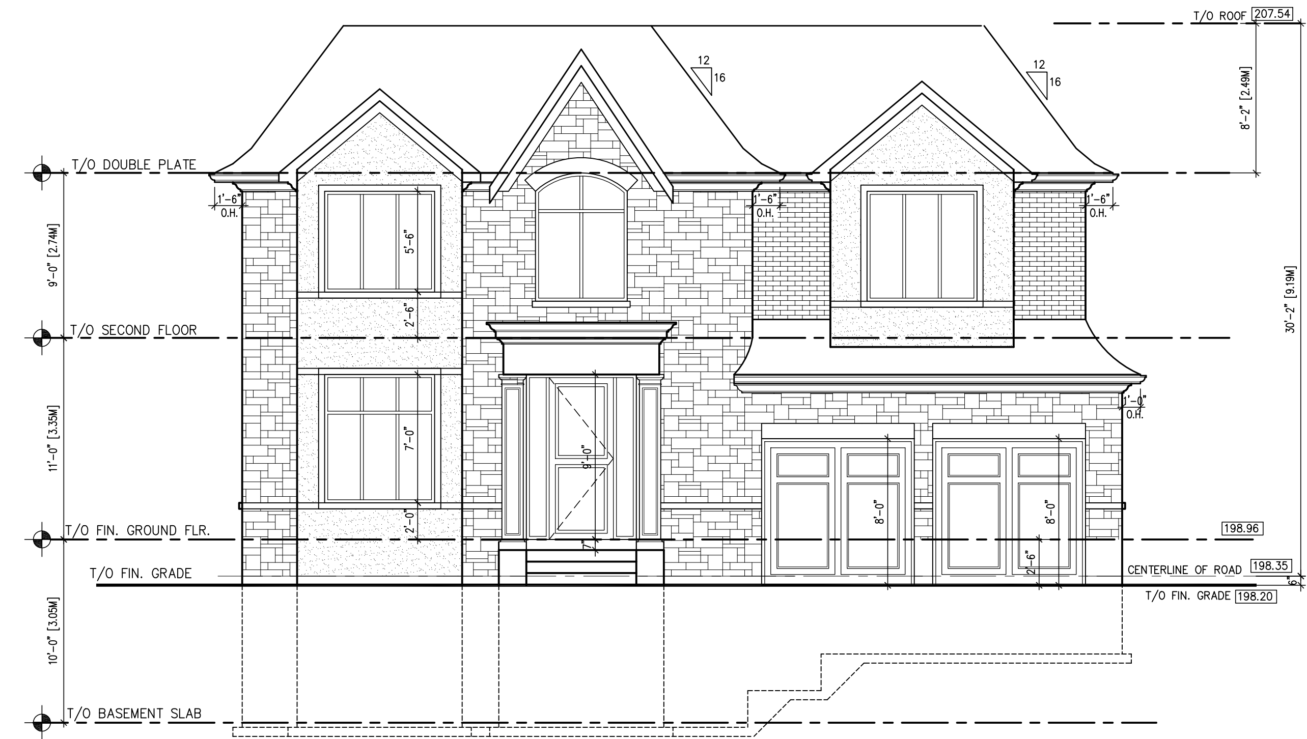
1 WEST SIDE ELEVATION SCALE: 3/16"=1'-0"
