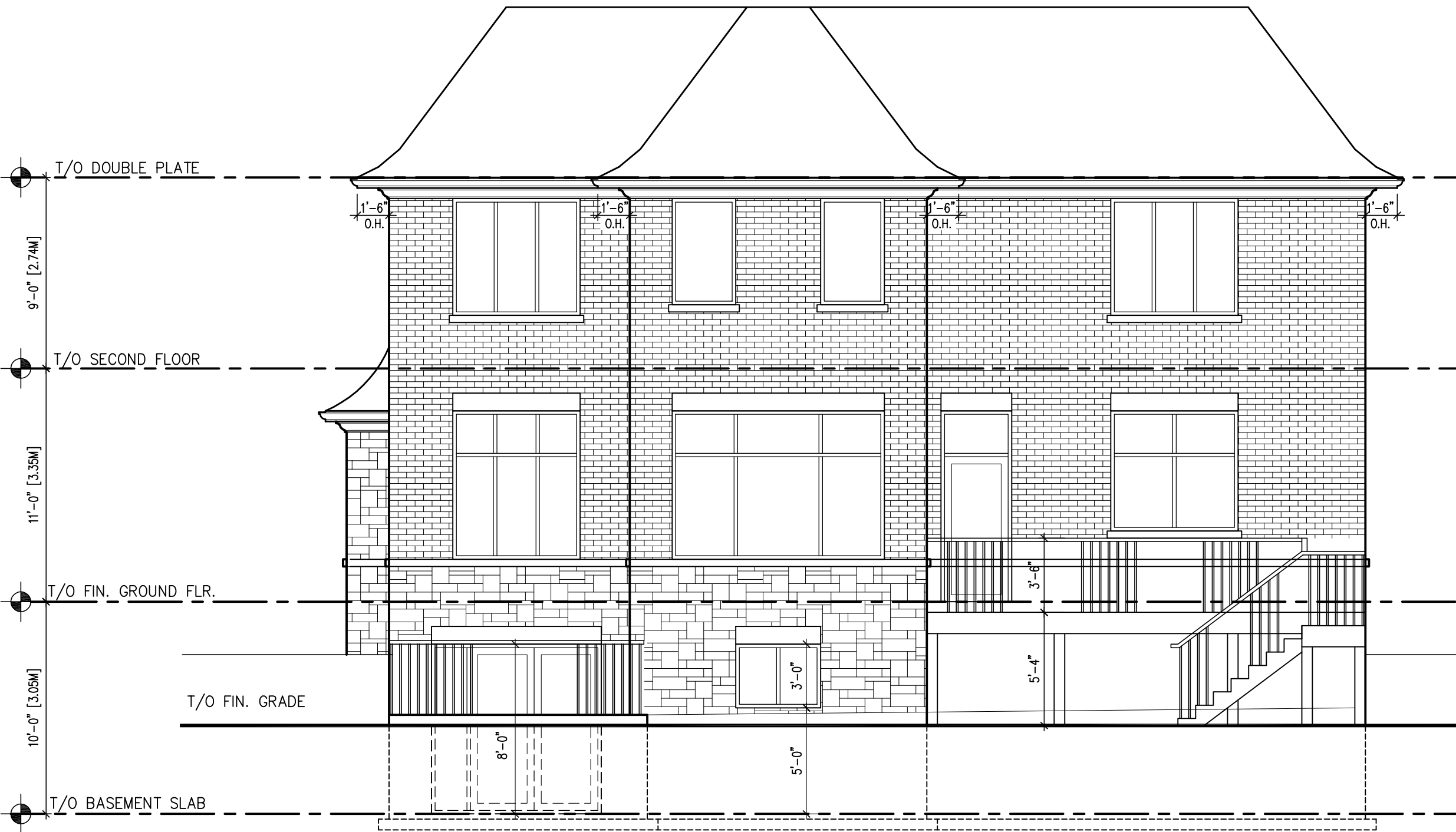
3 EAST SIDE ELEVATION SCALE: 3/16"=1'-0"
